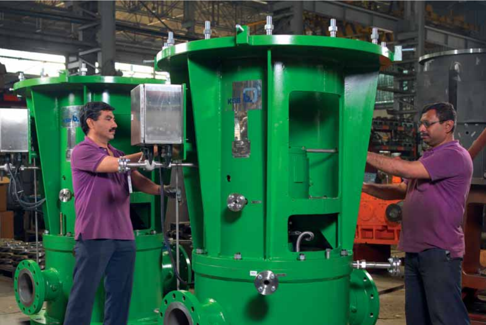
Vertical high-pressure inline pumps WKT pumps - Finishing touches before despatch at Power Projects Division, Chinchwad, Pune.
